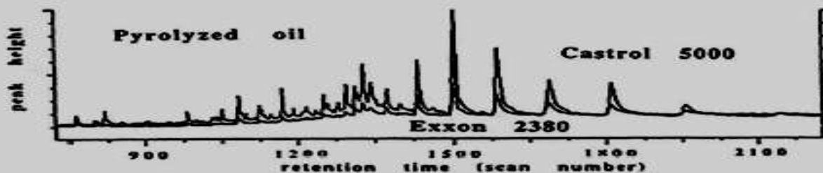
FIGURE 1 Gas chromatograph scans of two turbo jet engine oils and their volatile products produced at 525°C.
