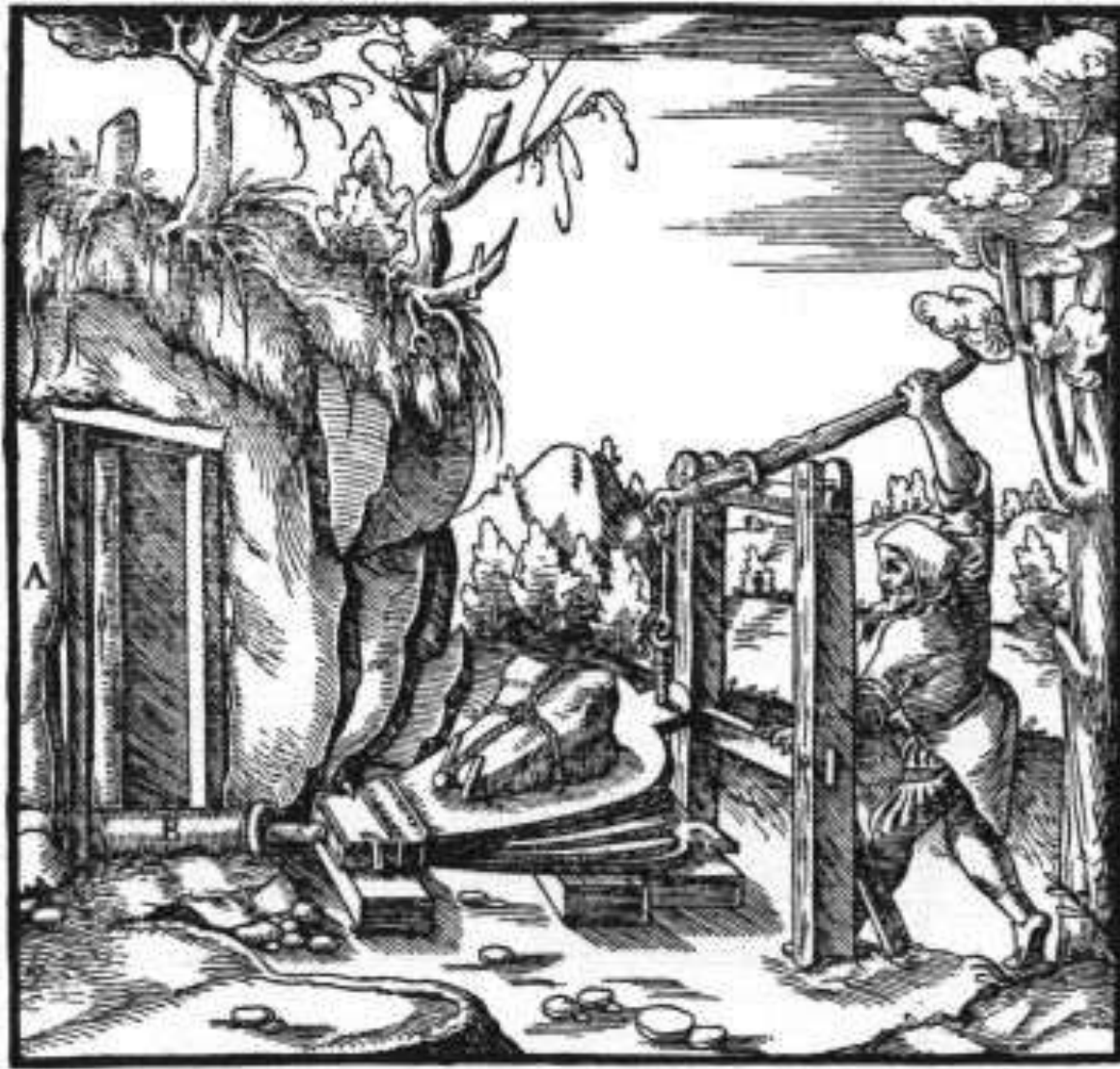
A—TUNNEL. B—PIPE. C—NOZZLE OF DOUBLE BELLOWS.
